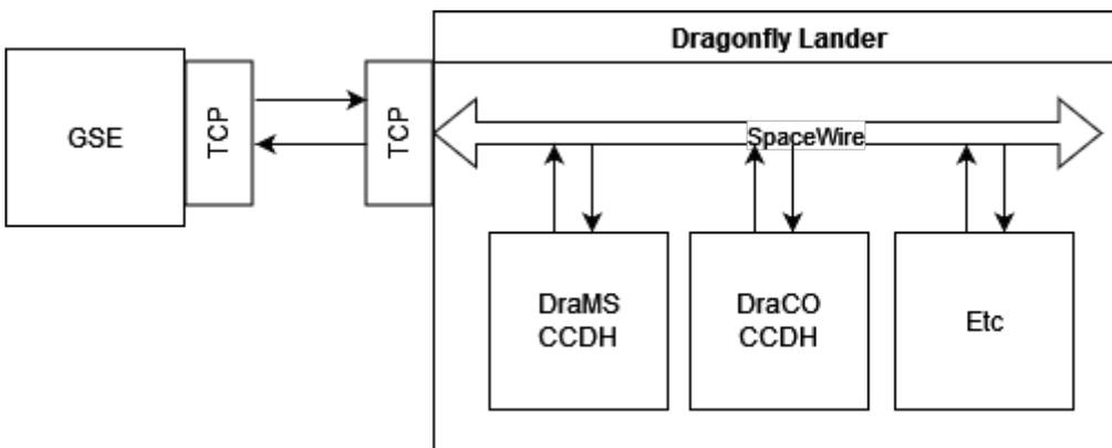
The SpaceWire connections can be simulated in software or replaced with a dedicated SpaceWire device (either the "Microtel box" or the "STAR-Dundee Brick").
